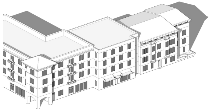
Figure 5.4 A long building facade can be broken into smaller modules and include slight shifts in the wall plane. Standards for an active ground floor help achieve a livelier, more welcoming streetscape and prevent a long and monotonous building facade with no entrances.
